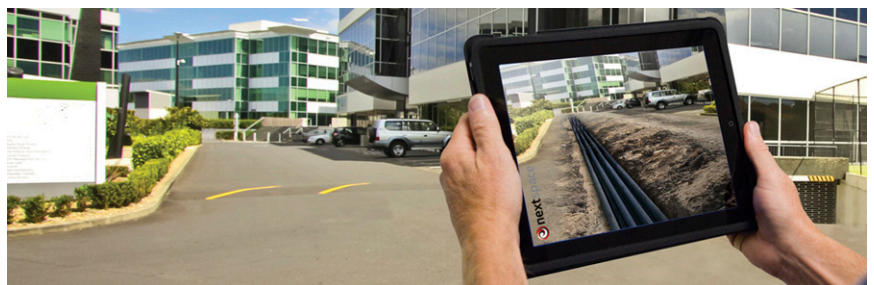
Fig. 1. Handheld consumer devices such as this tablet computer can augment a real scene with data obtained from Digital Earth, such as these underground pipes. (Image courtesy of NextSpace.)
