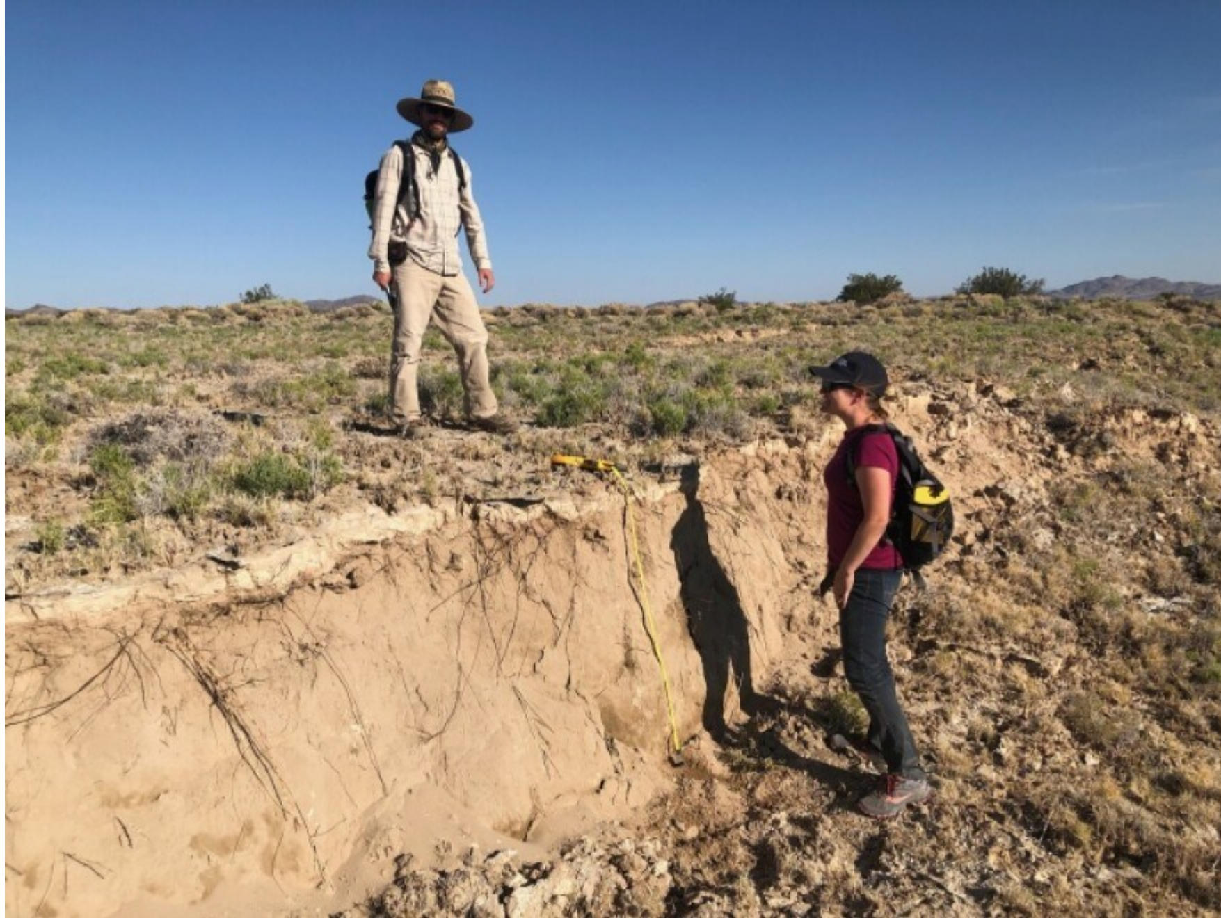
California Geological Survey geologists, Ellie Spangler and Nick Graehl, measure 3.75 feet of uplift at the Naval Air Weapons Station China Lake. (Courtesy of Brian Olson)
