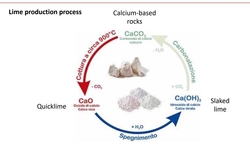
The quality of the lime depends on the **type of stone** burned and on the **duration and temperature** of firing
