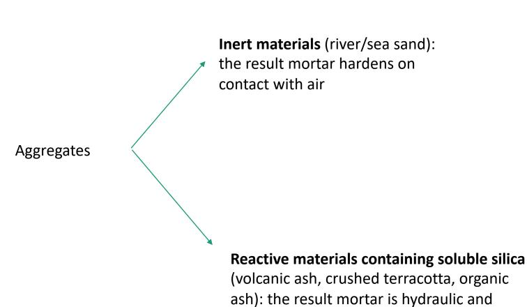
ash): the result mortar is hydraulic and hardens by means of a chemical reaction which requires water
