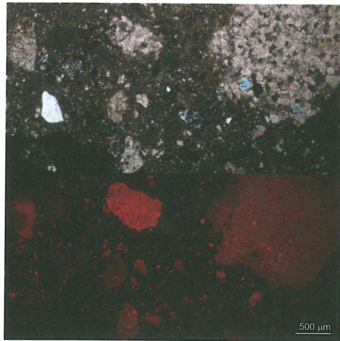
Fig. 5.3: Above: polarized optical microphotograph of a thin section of an historical mortar (crossed Nicols), clearly showing polycrystalline geologic carbonate embedded in the mortar matrix. Below: the same area measured in cathodoluminescence spectroscopy. The orange luminescence clearly shows that geologic carbonate is present both in large fragments as aggregate and as fine particles intermixed with the mortar binder.
