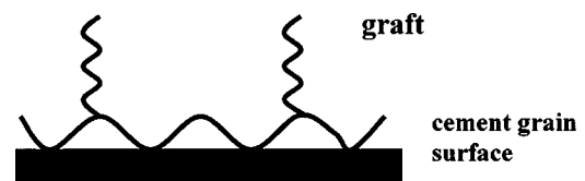
Fig. 12. Schematic description of adsorbed graft polymer superplasticizer causing steric hindrance (adapted from Haneharo and Yamada 1999)
