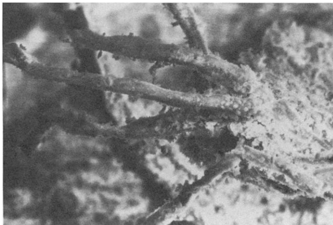
Figure 12. Scanning electron micrograph of fibers used to strengthen the Nahal Hemar sculpture by forming a fiber-plaster matrix composite. Particles of lime plaster are seen adherent to the fibers (350×).
