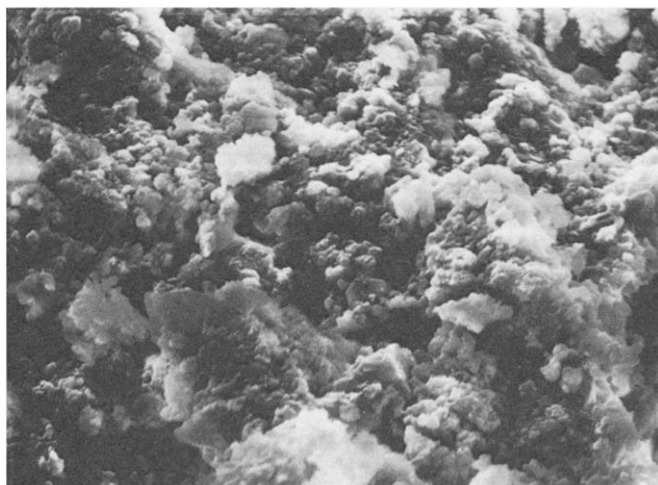
Figure 7. Microstructure of a Tel Ramad Vaiselle Blanche (whiteware vessel) illustrating the lime plaster structure (2700 \times ).
