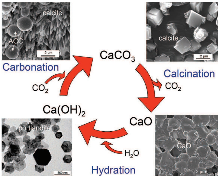
Fig. 4. The lime cycle: Electron microscopy images show reactant and products of the different stages of the cycle. ACC: Amorphous Calcium Carbonate.
